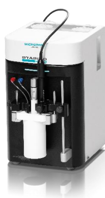
Figure 1: (a): STABINO ZETA (b): Zeta potential calculated from relative displacement of the ion cloud measured at a voltage, U (streaming potential)
